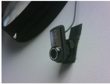
This is a tiny, inexpensive camera (2 1/4" high!), but it does 640x480 resolution video at 30 frames per second, so it does what we need. I would now spec the Logitech QuickCam Pro 9000, which would be easier to wall-mount (I ended up using Velcro here). Since it's on the opposite side of the room from the computer, I had to daisy-chain a couple of powered USB extension cables to reach. (Belkin 16.4' USB Active Extension Cable, F3U130-16).
