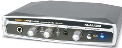
(You may notice the "phantom power" indicator; these condenser mics need a 48 volt power connection to work.) The MobilePre powers the mics, takes the signals, and converts them to digital signals which get to the computer via a USB cable.
